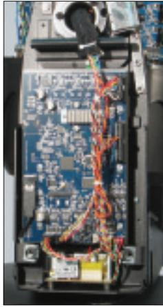
Fig. 20: Motor Driver Board.
