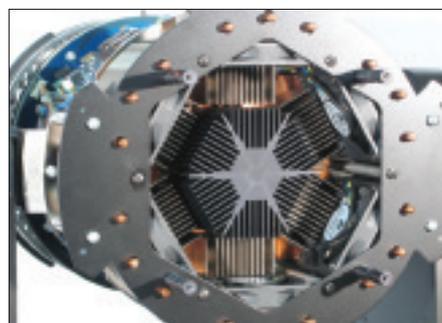
Fig. 7: Heat Sinks and Fans.
