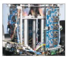
Fig. 4: Driver Boards and Light Pipes.
