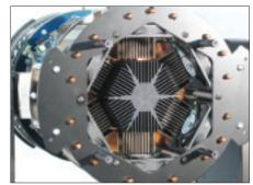
Fig. 7: Heat Sinks and Fans.
